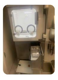
Integrated airborne surface disinfection unit (ASD), using non-wetting fog technology.
